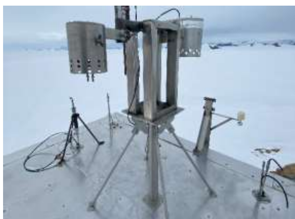
Image left: auto-sampler for organic analyses on the southern science shelter at PEA; image right: new installed auto-sampler for VOC near the coast
