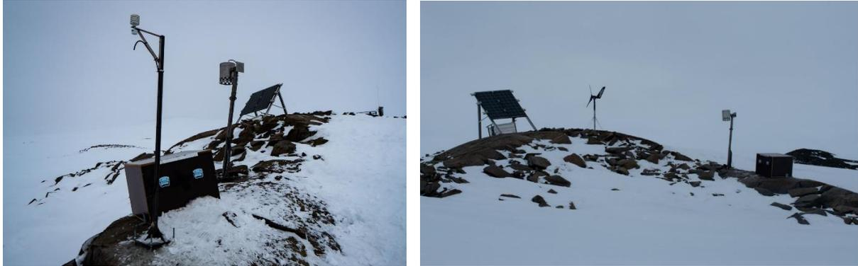
Figure 2: View of the installation at the CLIMB remote site; left image, from left to right: the pole with the meteorological data logger and the inlet for the optical particle sizer (OPS) attached to it; below the box with the OPS inside and other controlling devices for the VOC sampler and power control, in the middle the pole with the VOC sampler and the solar panel; right image: the wind turbine can be seen and another power-control-battery box under the solar panel
