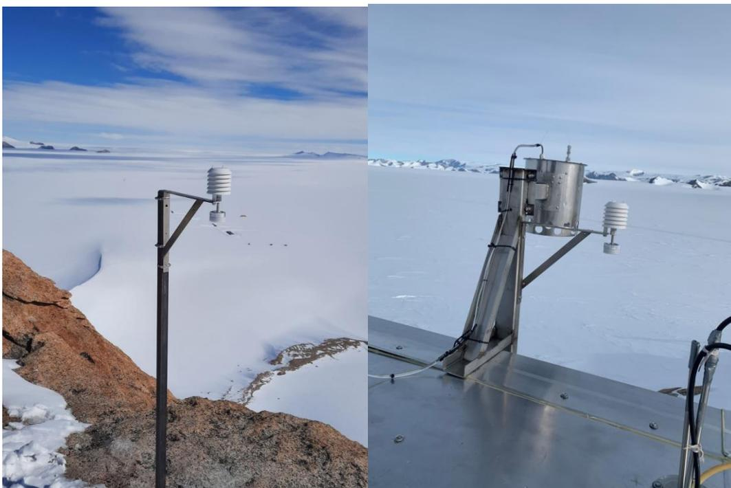
Figure 10: the meteorological data loggers on the Utsteinen nunatak (left) and on the southern science shelter (right)
