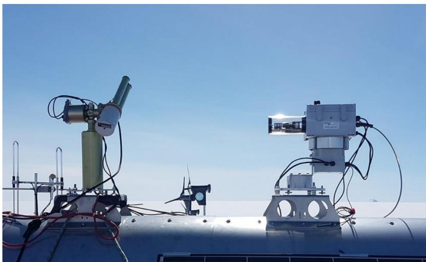
Figure 5: The CIMEL sunphotometer (Left) and Airyx MAX-DOAS (Right) on the roof of the PEA station.
