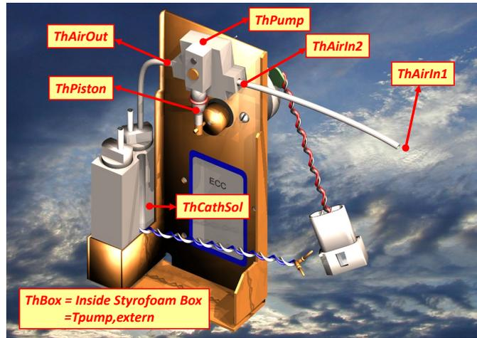
1. For balloon borne electrochemical concentration cell (ECC) ozonesondes an accurate measurement of the pump temperature is essential for accurate ozone measurements.
