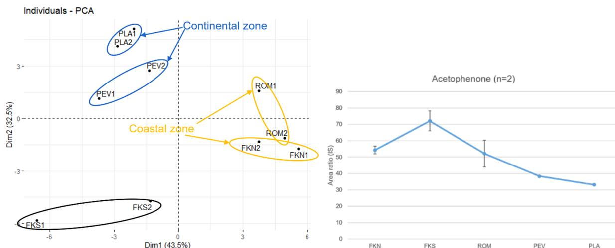
Figure 2: PCA analysis of the GC-MS data obtained from Tenax TA tubes exposed during one year from Nov/Dec 2017 to Nov/Dec 2018 on the left. Response of acetophenone (oxidation product of ethylbenzene) relative to the internal standard (toluene-D8) for different sample sites on the right.
