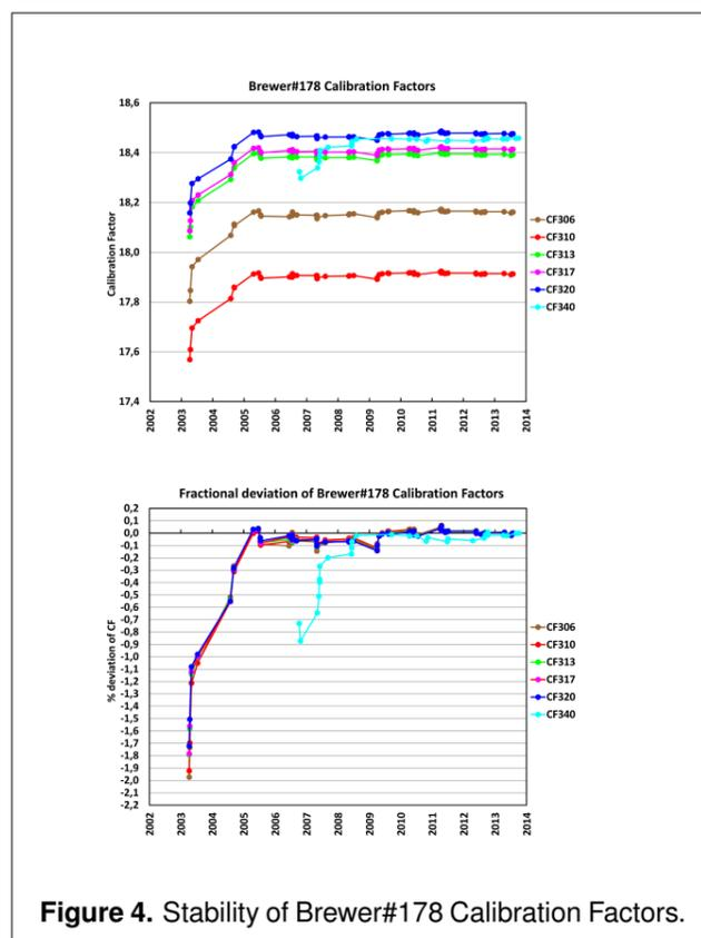
Figure 4. Stability of Brewer#178 Calibration Factors.
